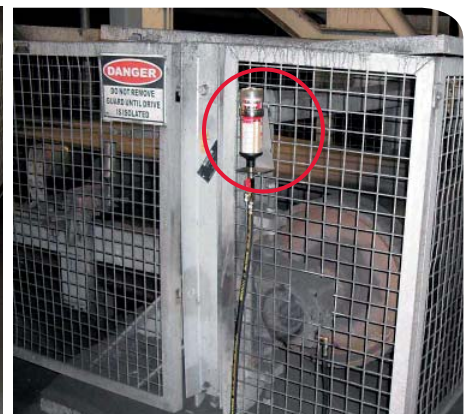
Lubrication system: perma STAR VARIO with LC 250 cm 3
